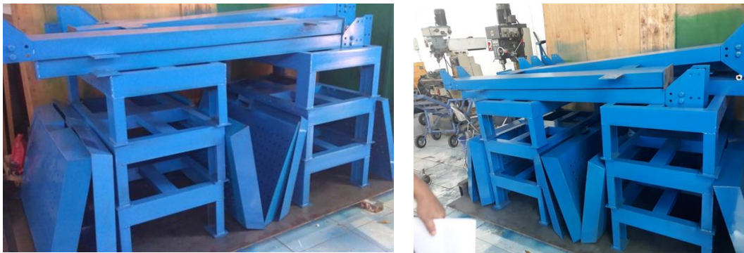
Gambar 6. Proses knock down alat press hidrolik multi gawang
