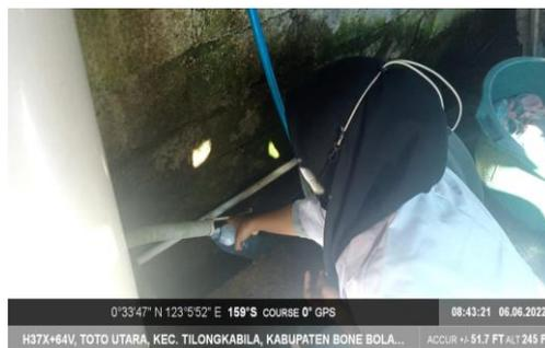
Gambar 1 Proses sampling air limbah laundry di Naya laundry, Kec.Tilongkabila, Kab. Bone Bolango, Gorontalo
