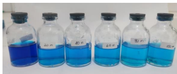
Figure 7. Adsorption of methylene blue with magnetite based on reaction time
