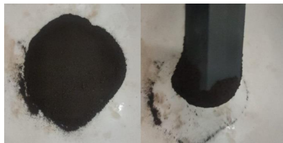
Figure 2. Magnetite synthesis results ( \text{Fe}_3\text{O}_4 ) and testing using a magnetic bar
