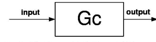
Gambar 2. Diagram Blok Pengendali Proporsional
