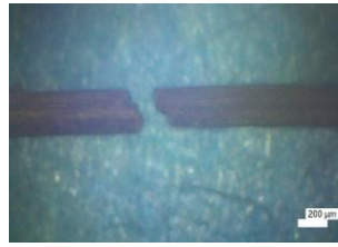
Gambar 6. Foto mikro patahan brittle fracture axial split (keras-getas) 2% NaOH
