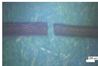
Gambar 8. Foto mikro patahan independent fibrillar 8% NaOH
