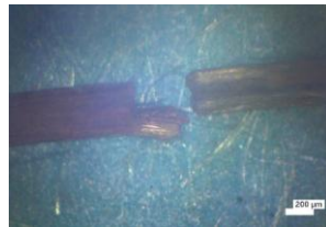
Gambar 7. Foto mikro patahan ductile dan stake socket 5% NaOH
