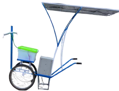
Gambar 5. Alat portable spray berbasis panel surya
