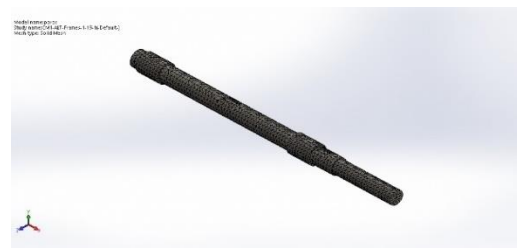
Gambar 3. Meshing Poros Roda
