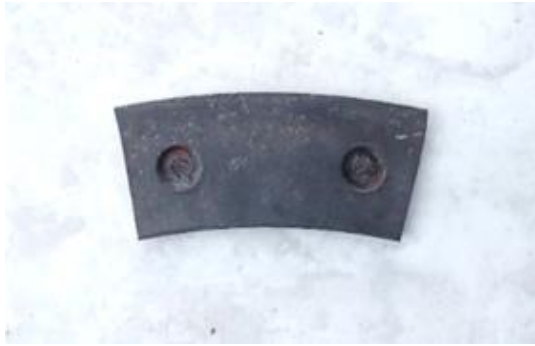
Gambar 1. Brake Lining Pesawat Cessna Grand Caravan 208B
