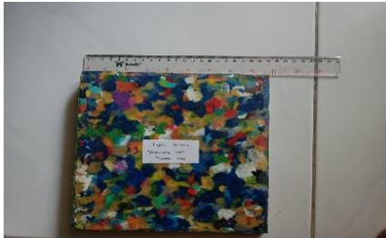
Gambar 3. Hasil Proses Compression Moulding
