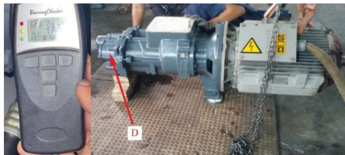
Gambar 9. Pengukuran shock pulse bearing screw D.
