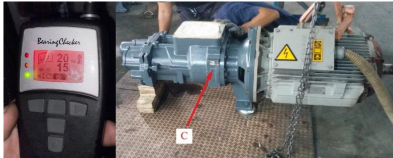
Gambar 8. Pengukuran shock pulse bearing screw C.
