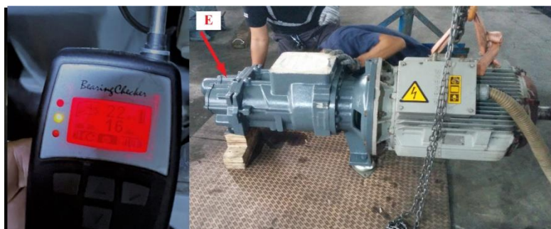
Gambar 10. Pengukuran shock pulse bearing screw E.
