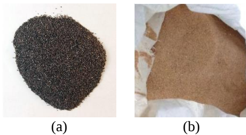
Gambar 2. (a) material abrasif aluminium oxide, (b) material abrasif pasir silika
