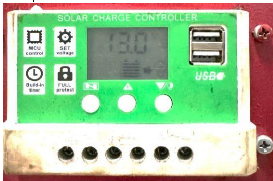
Gambar 12. Solar charger controller
